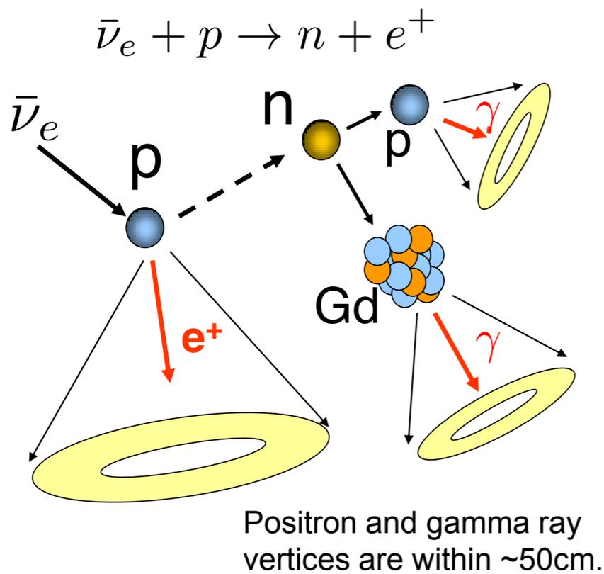
Neutron tagging in Gd-enriched WC detector (Super-K with 100 tons Gd to trap neutrons).
